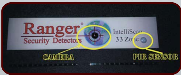
Motion Detection Camera The camera is triggered every time it senses a movement. The movement is detected through the PIR sensor, which is mounted on the back of the header next to the camera.
